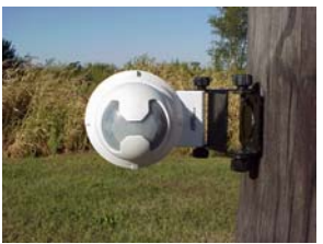
Front view of normal direction of detection lens placement. Arrows on lens pointing parallel to ground (horizontal) with long range pattern.
