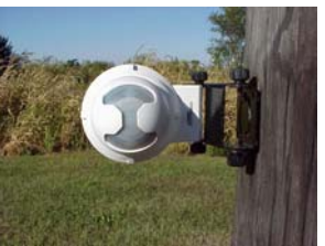
As experimentation, you may want to try rotating the lens assembly so arrows are pointing up and down (vertical) with long range pattern.
