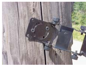
Mount sensor on backside of pole and allow room to pivot bracket in semi circle slot holes for final adjustment. (Model 1000V shown) Model 1000 no bracket with unit.
