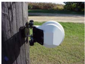
Notice level view of sensor to driveway at about a 3 ft. height mounted behind the pole.
