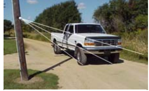
You can also mount the sensor higher to control the length of the beam to a shorter more pinpointed distance.
